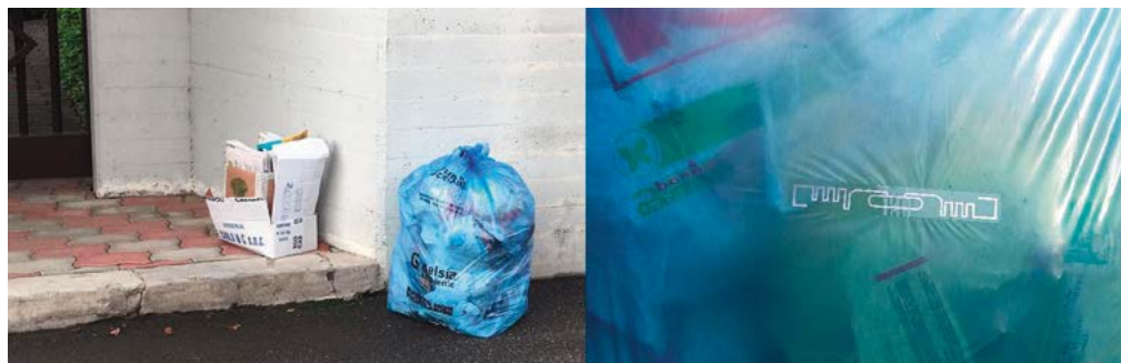
FIGURE 8. Example of visibility, proximity & identification with translucent bags for the “residual waste” fraction & RFID tags in Seveso (Italy) (©2018waste4think)
